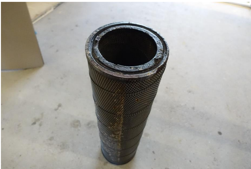
Filter from a heat pump screw compressor oil separator running with air and water and possibly other contamination in a very chemical reactive system.
